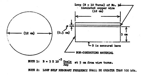
Figure 1 - Loop used for radiating magnetic fields.
