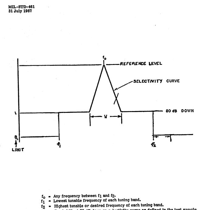
W = Bandwidth at 80 dB down on solectivity curve as defined in the test sample technical requirements or the control plan.
